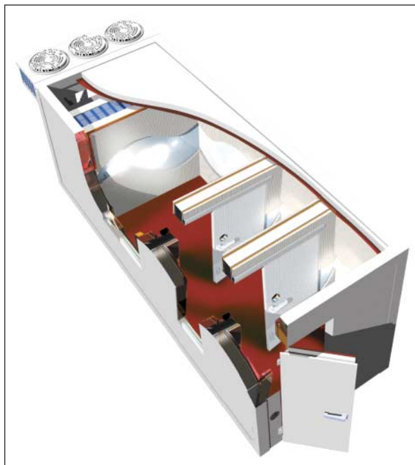
Figure 1. Sketch of the Uniers Cryo-Combi whole-body cryotherapy device (Oy MJG Uniers Ab, Helsinki, Finland) showing the 3 chambers.
