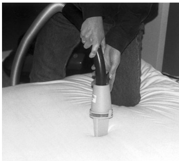
Fig. 2 ALK sampling nozzle
