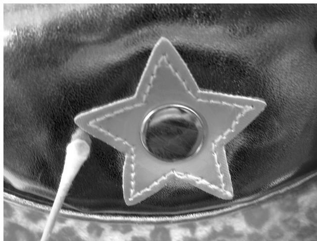
Figure 2. A snap on a child's toy purse was found to contain nickel by dimethylglyoxime testing.
