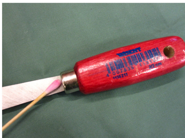
Fig. 2. A positive dimethylglyoxime (DMG) test result indicating nickel release from a metal ring located at the end of the grip, that may cause nickel allergy and dermatitis.
