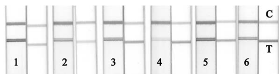
Fig. 3 LFIA results of wiped filter extracts. Samples were taken in an animal facility in Germany (Table 1). After extraction of the samples, eluates were applied to both a RUA (left membrane) and a MUA (right membrane) LFIA. Table 1 shows a comparison between LFIA results and allergen levels of the extracts obtained with EIA. The upper line (C) of each test: control line, the lower line of each test (T): test line.
