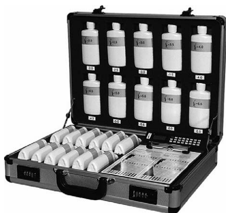
FIG 6. STT. Concentrations of PEA, ranging from 10^{-2} to 10^{-10} log vol/vol in half-log concentration steps, are provided, along with blanks for forced-choice testing. Photo courtesy of Sensonics, Inc. © 2000 Sensonics, Inc.
