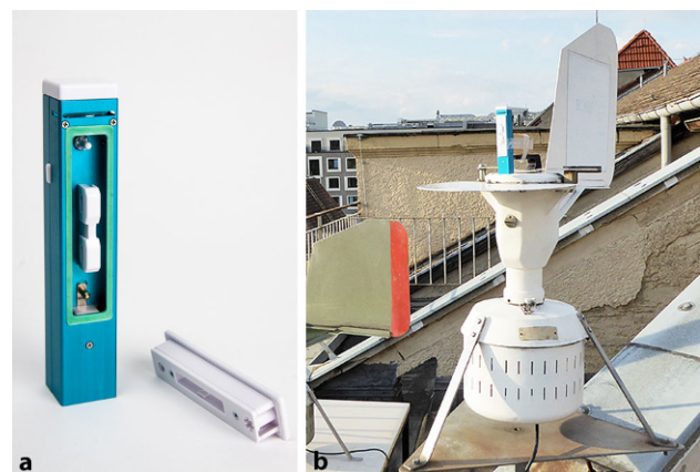
Fig. 1 a The Pollator with exchangeable cartridge. b The position of the Burkard trap and Pollator for comparative measurements
