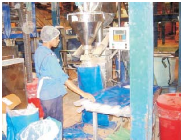
Fig. 2. A spice mill factory where spices are milled, blended and packed generates high levels of inhalable dust, which poses a health risk to exposed workers.
