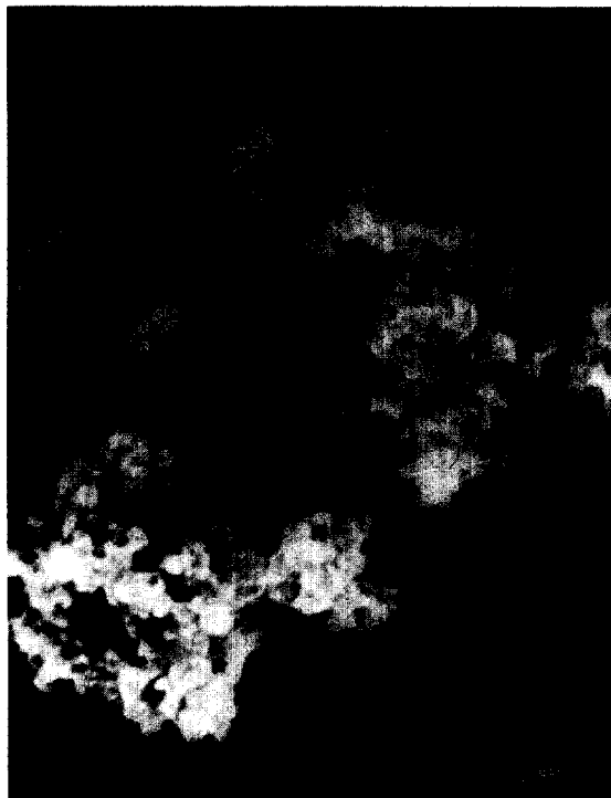
FIG. 1. Scanning electron micrograph of particulates emitted from diesel engine (original magnification \times 30,000 ). The samples were dusted onto double-sided sellotapes and coated with platinum films. The acceleration voltage was 25 kV.
