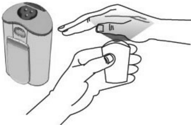
Figure 1 The Vein Locator-Universal transillumination device and method of use.
