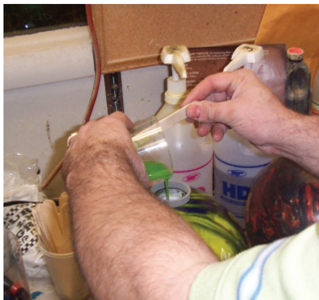
Figure 5. Bowling ball plugging, step 3: pouring the epoxy into the bowling ball hole.
