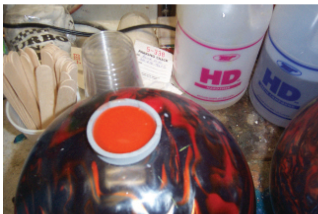
Figure 7. Bowling ball plugging, step 5: the hole of the ball is plugged and ready to cure for 12 hours.
