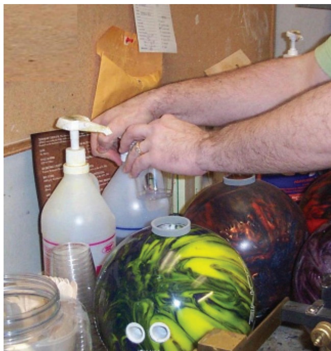
Figure 3. Bowling ball plugging, step 1: filling a clear plastic cup with a two-part epoxy resin/hardener. Note the lack of use of protective gloves.
