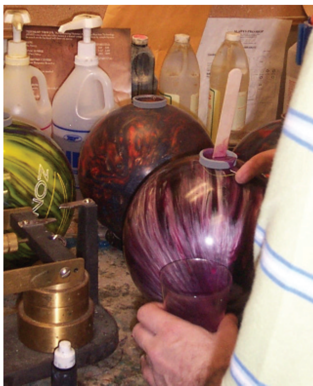
Figure 6. Bowling ball plugging, step 4: wiping away excess epoxy resin with a bare finger.
