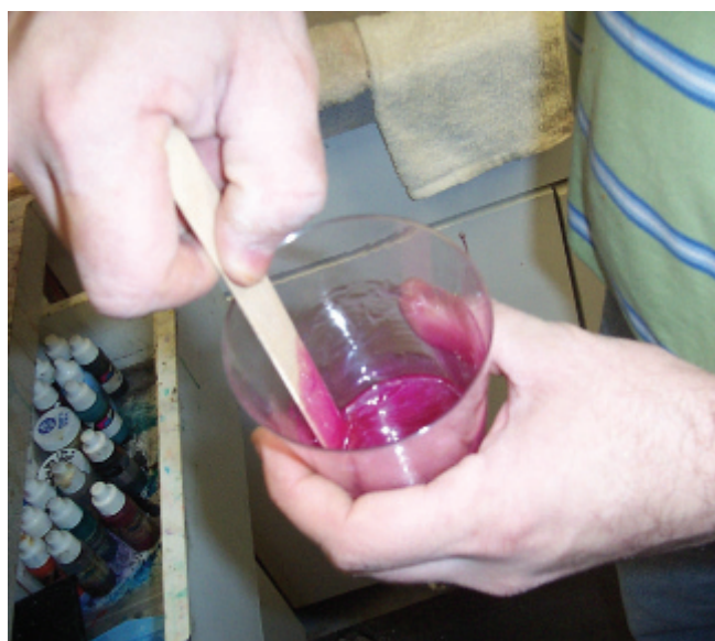
Figure 4. Bowling ball plugging, step 2: mixing the epoxy compound by hand.
