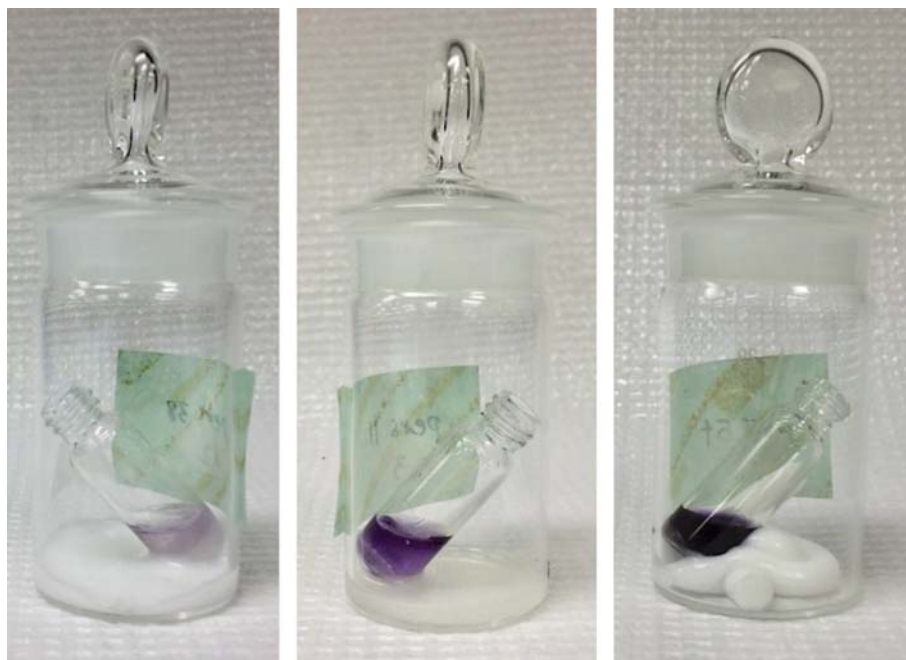
Figure 2. Examples (from left to right) of products with mild, moderate, and strong formaldehyde release.
