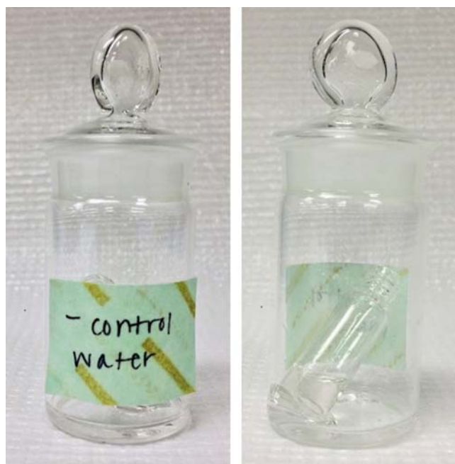
Figure 1. Front and back views of a 30-mL stoppered bottle with 1 mL of a product (in this case, distilled water as a negative control) at the base and an uncapped small vial containing a reagent solution.
