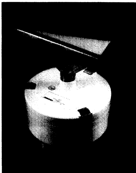
FIG. 1. The Air-Sentinel, a volumetric air filtration device expressly designed for collection and quantitation of indoor airborne antigens.
