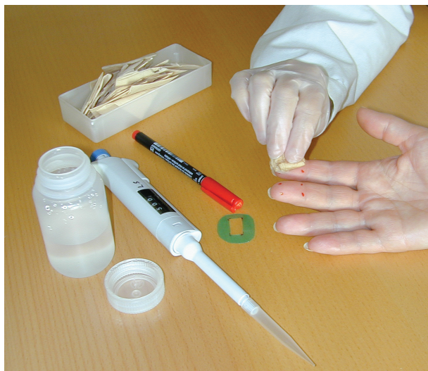
Fig. 1. Acid wipe sampling for assessment of nickel, chromium and cobalt deposited on skin.
