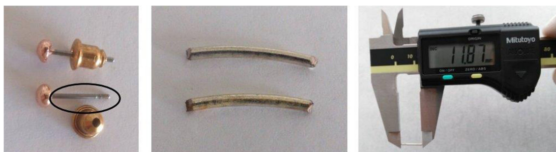
Fig. 2 Preparation steps of samples: after labelling and cutting the penetrating part and calculation of surface area by a caliper
