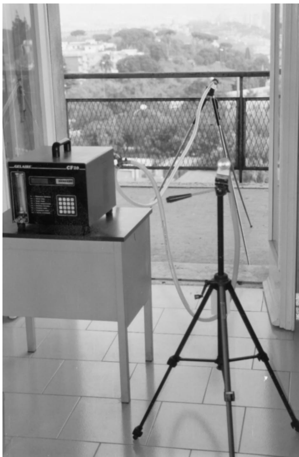
Figure 1. High volume air sampler (CF/20 Gelaire, Flow Labs, Milan, Italy) with the modified double tube, each with one filter, so that one tube and one filter are outside the room (in this figure with open balcony) and the other tube and filter are inside. Both operate at 10 L/min.
