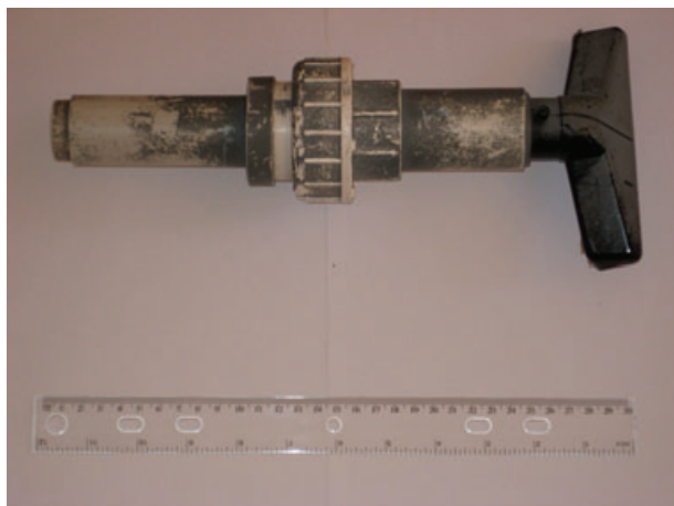
Figure 1. Polyvinyl chloride collection apparatus attached to end of the telescopic rod of the vacuum cleaner for dust sample collection.
