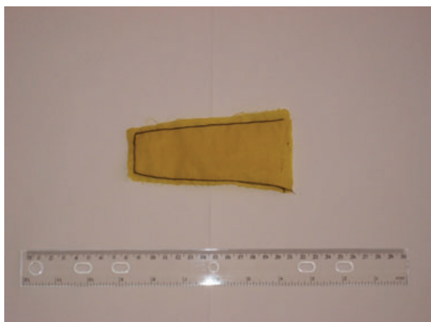
Figure 2. Conical cloth filter to fit inside PVC collection apparatus to trap the dust sample.
