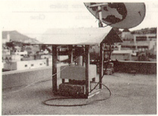
Fig. 1. A rotorod sampler installed on the roof top of an apartment.
