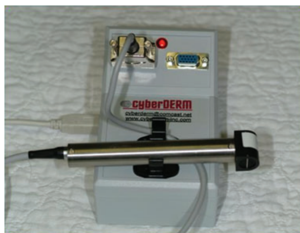
Figure 1. The DermaLab ® Open-Chamber Evaporimeter consists of a cylindrical hand-held probe with paired sensors in a diffusion chamber which measures relative humidity and temperature when placed perpendicular to the skin surface. The vapour pressure gradient in the chamber is used to calculate evaporated water loss over a constant skin area.
