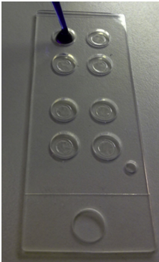
Fig. 1. Picture of the multiwell system used to compartmentalize eight hydrogel plugs. The hydrogels are made of a DMA-Bis solution (4% T, 3% C) that can be desiccated and rehydrated in 60 min by adding 30 \mu L of solution.
