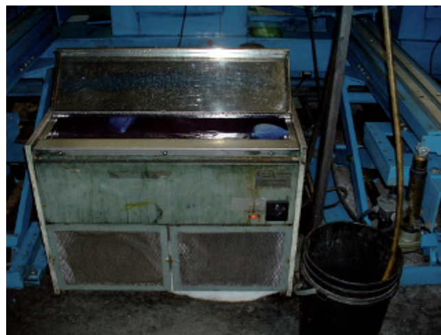
Figure 1. Fountain solution collection drum dedicated to the worker's press only.
