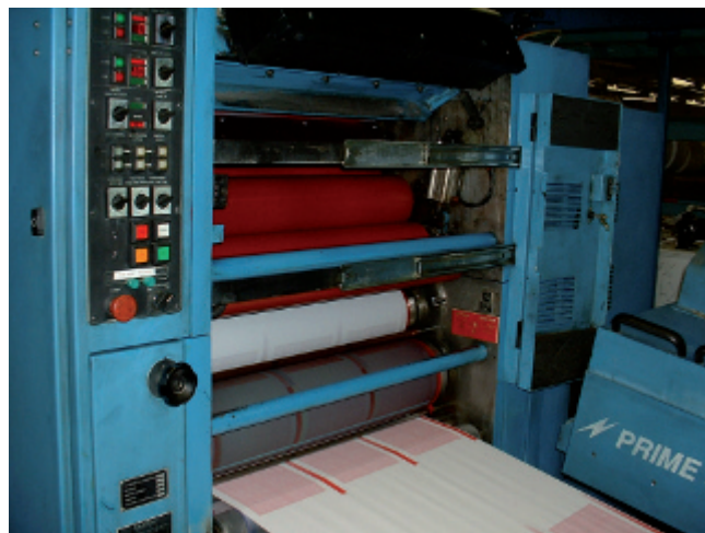
Figure 4. A print deck with the blanket (roller) and plate cylinders visible. Following a print run, the blanket is washed by the worker.
