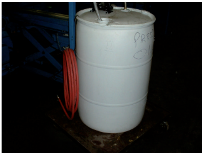
Figure 2. Fountain solution reservoir.
