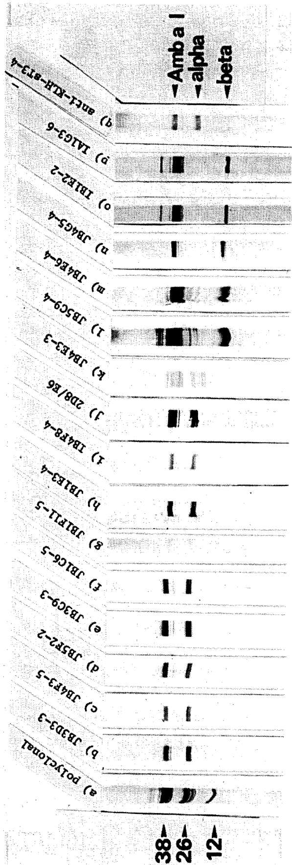
Fig. 2. Binding patterns of 15 anti-denatured Amb a I MAbs to "Western" blots of pp Amb a I after SDS-PAGE show their specificities for Amb a I (38,000 mol. wt) and their localizations to the alpha chain (26,000 mol. wt) or beta chain (12,000 mol. wt) of Amb a I. Fifty \mu l of pp Amb a I (150 \mu g) were separated on SDS-PAGE using a modified Laemmli technique (Laemmli, 1970) with a 20% acrylamide resolving gel and a 3% acrylamide stacking gel. After blotting to nitrocellulose, immunochemical specificities of individual MAbs were determined by subsequent incubations with MAb supernatants diluted 1:10, the appropriate subclass specific AP-labeled goat anti-mouse Ig, and an NBT/BCIP substrate system. Lane a was probed with polyclonal serum (1:100 dilution) from a mouse immunized with r&a Amb a I and boosted with pp Amb a I. The MAbs in lanes b-j are alpha chain specific while those in lanes l-p are beta chain specific. Lane q was probed with polyclonal serum from a mouse immunized with KLH-sTs-4 and shows the alpha chain specificity of this antiserum.
