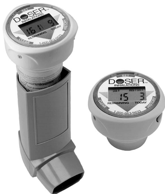
FIG 1. Doser attached to top of MDI ( left ). Display shows daily total and doses remaining in MDI inhaler canister. Face of Doser showing recent history of use of attached MDI ( right ).
