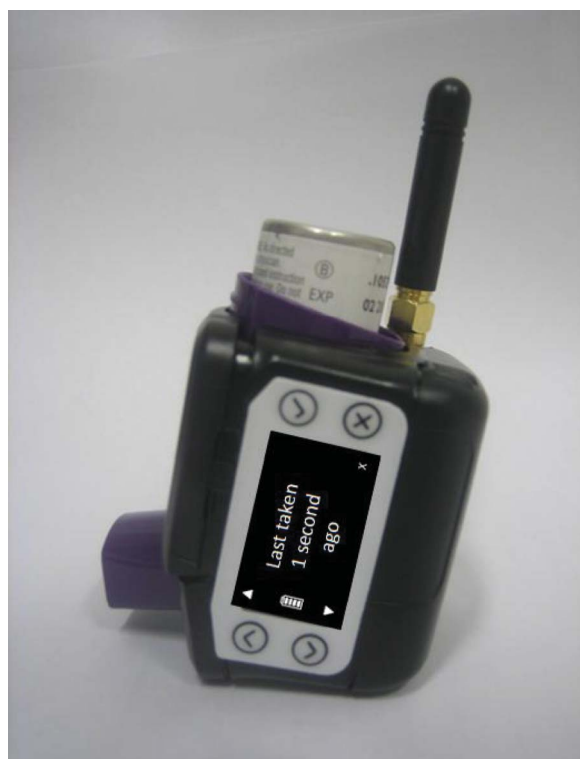
FIGURE 1.—Seretide™ pMDI inside a ST in reminder mode with adherence feedback: “Last taken” is displayed on the start screen, stating time since last actuation.
