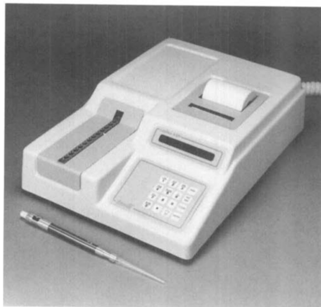
Figure 3. Labdex ASR TM automated strip reader spectrophotometer for reading the 12-well microstrips. To illustrate size, a small micropipette is shown in front of the instrument. A 12-strip well is in place for assay in the front left-hand portion of the instrument. The paper printout is seen in the right rear area. The keypad contains labeled keys for initiating the various procedures.
