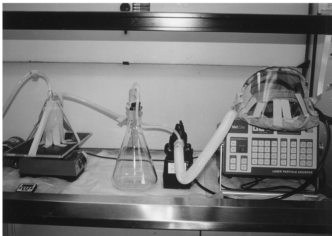
Figure 2. The HEC challenge apparatus in an externally ventilated fume hood.
