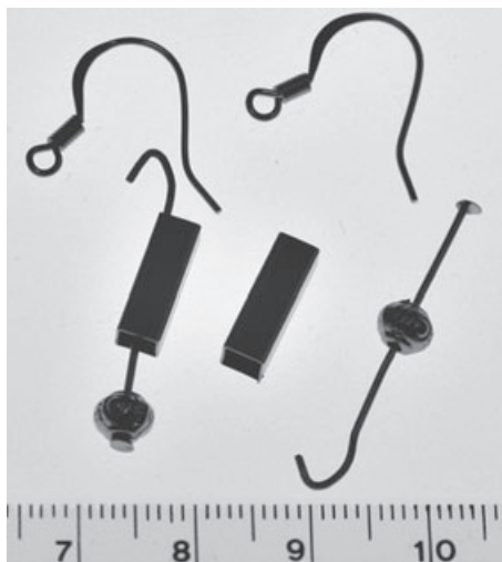
Fig. 3. A pair of earrings has been dismantled prior to area measurement. Both the interior and the exterior of the square tubes in the lower part of the figure were included in the total area as these will become exposed to artificial sweat during chemical analysis.
