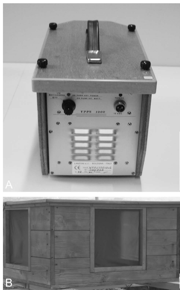
Figure 1. Pollen trap VPPS 1000 (A) [ 20 \text{ cm} \times 30 \text{ cm} \times 25 \text{ cm} , width ( W ) \times length ( L ) \times height ( H )] located inside the 'confinement simulator' (B) ( 100 \text{ cm} \times 150 \text{ cm} \times 60 \text{ cm} , W \times L \times H ) on the roof of the Agriculture Faculty of Perugia University, Italy.
