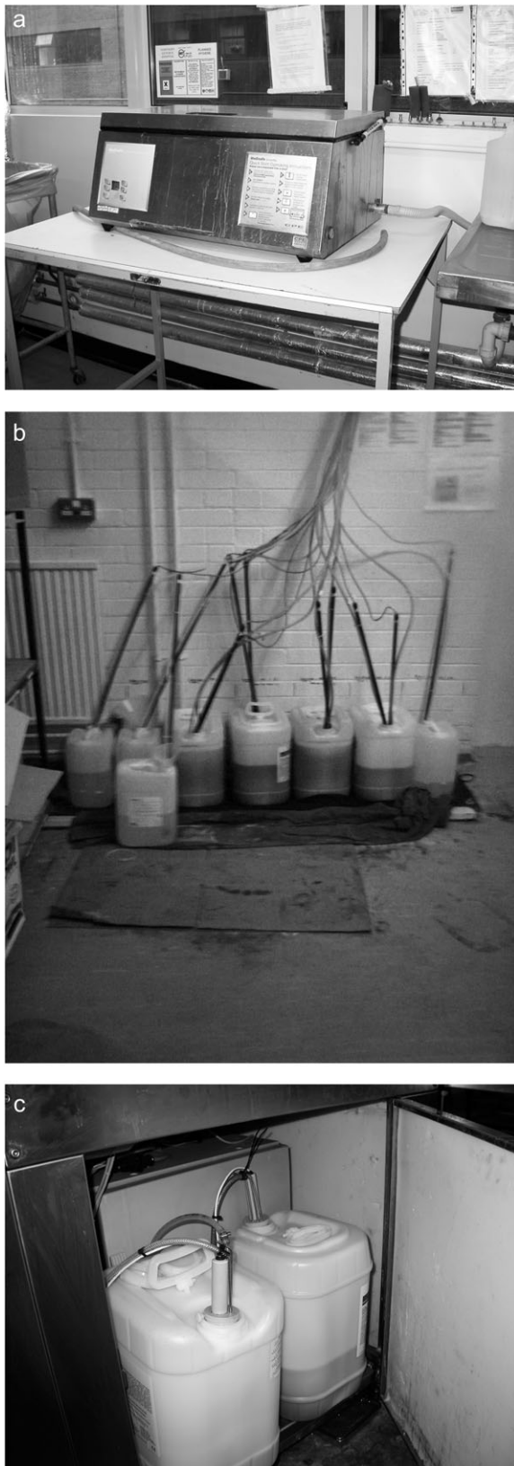
Figure 1. (a) An ultrasonic bath for cleaning surgical instruments. (b) The area for volumetric dosing of enzymes (note: absorbent material had been used to catch spilt chemicals). (c) Enzyme containers inside a surgical instrument washer drier machine.
