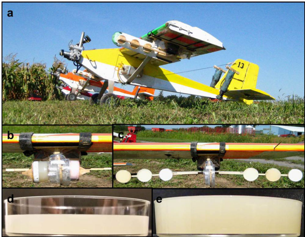
Fig. 1 Unmanned aerial vehicles (UAS) were used to collect colony-forming units of Fusarium spp. in the planetary boundary layer. UAS had a 3.0 m wingspan and were powered with a 50 cm 3 engine (a). Spore sampling devices were attached
