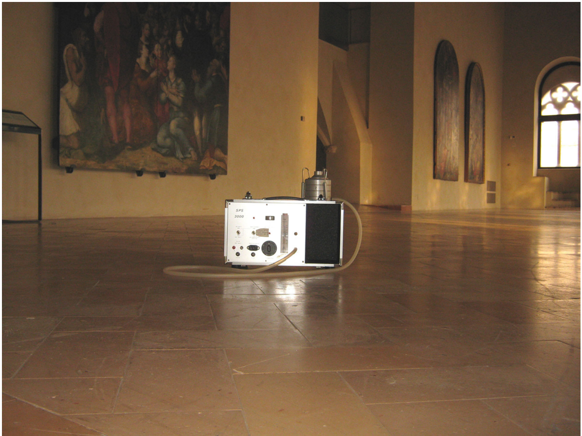
Fig. 1 Andersen Microbial Air Sampler in the Art Gallery of Perugia, Italy
