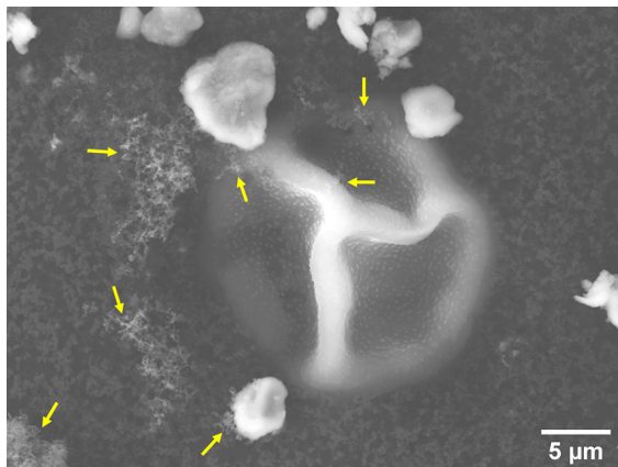
Fig. 3 Secondary electron image of a birch PG observed after exposure to outdoor air in the conventional HTS. The exine is partially covered with mineral dust particles (bright irregularly shaped supermicron particles) and soot aggregates (arrows point to clusters of carbon nanospheres arranged in a chain-like structure lying on the substrate and on the pollen wall)
