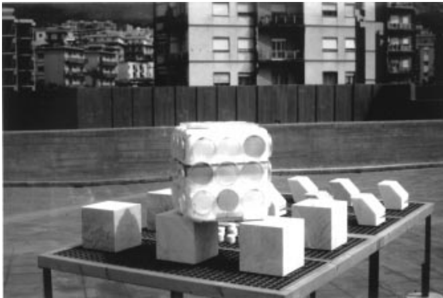
Figure 1. Exposure table located in the terrace of the Messina Museum on which marble blocks are placed. Polystyrene cube with Petri dishes containing different cultural media (in triplicate): DRBC, Oxoid; Glucose Mineral Agar, GMA, plus dichlorane addition, Czapek dox Agar, CZ, Oxoid.
