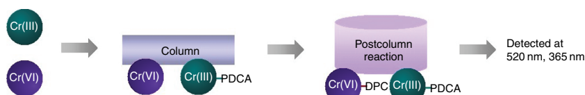
Fig. 1. Reaction on column and separation of Cr(III) and Cr(VI). DPC, 1,5-diphenyl carbazide; PDCA, pyridine-2,6-dicarboxylic acid.
