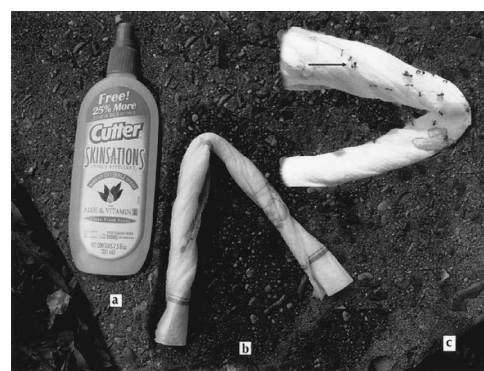
Figure 7. Paper towel test showing example of repellent tested (a), towel saturated with repellent (b), and ants stinging towel (c)
