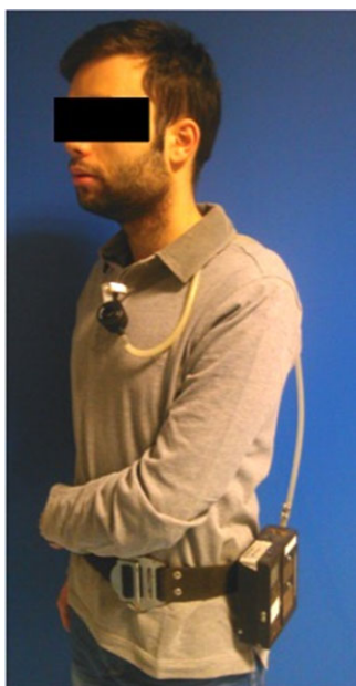
FIGURE 1. Woodworker wearing the IOM sampler connected to the air sampling pump. IOM = Institute of Occupational Medicine.
