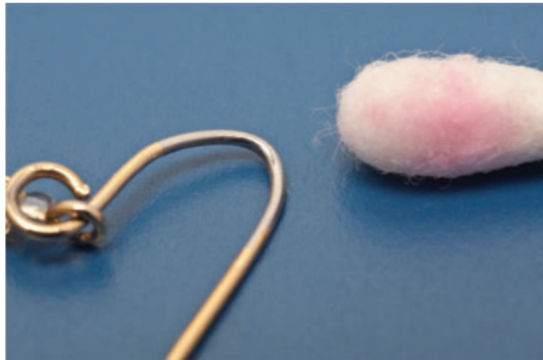
Fig. 1. Defective coating of an earring post resulting in nickel release as indicated by a positive dimethylglyoxime test result.
