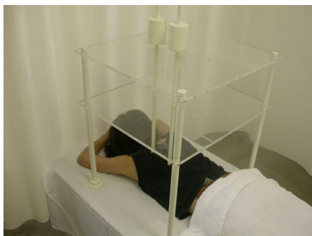
Fig. 1 Device for pressure challenge test (4 kg/1.5 cm 2 , for 15 min)
