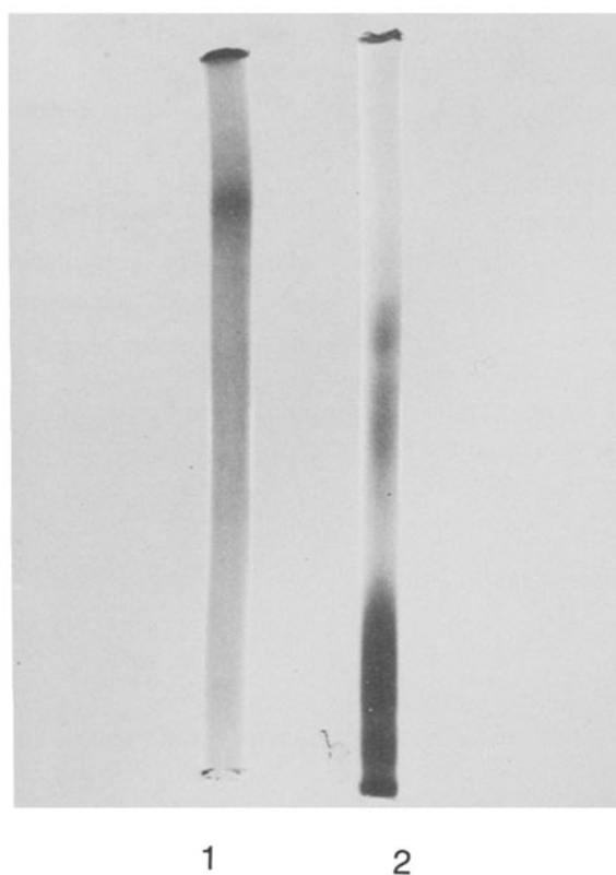
Plate 4. Polyacrylamide gel electrophoregram of vicilin subfraction of urdbean. 1, without SDS; 2 with SDS.
