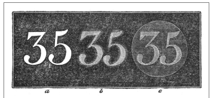
Fig. 3. Tulley's artificial test plate, which he used for assessing spherical and chromatic aberration. The degree of nebulosity indicates the degree of spherical aberration, and chromatic aberration shows in a fringe of colour mixed with the diffused borders. Reproduced by permission of the Syndics of Cambridge University Library [4].
