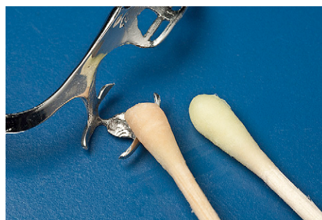
Fig 1. Left , cotton stick: positive test result of cobalt spot test indicated by red coloration. Right , cotton stick: reference as indicated by yellow coloration, that is, when cobalt spot test is negative and no cobalt is released.
