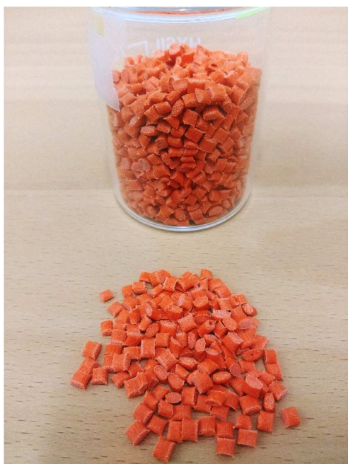
Figure S2. Orange polyamide pellets used for chain saw body covers.
