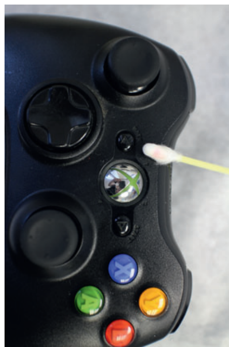
Figure 1. Xbox on dimethylglyoxime testing.
