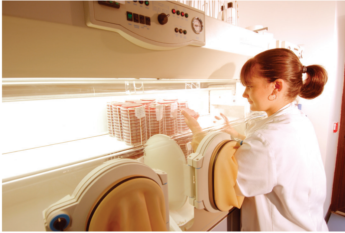
Fastidious anaerobic bacteria are readily killed by exposure to atmospheric oxygen. Here anaerobic culture plates are examined within an anaerobic cabinet
