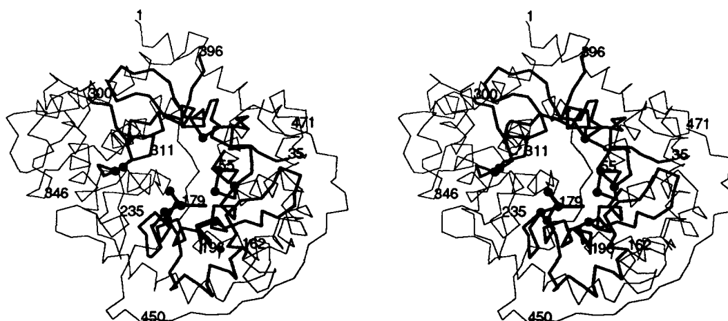
FIG. 6. Stereo view of an \alpha -carbon plot of glucoamylase-II(471). Positions marked with solid circles represent sites of directed mutation and/or chemical modification that result in significant changes in catalytic activity. Bold lines represent the five regions of sequence similarity observed amongst glucoamylases from Aspergillus .
