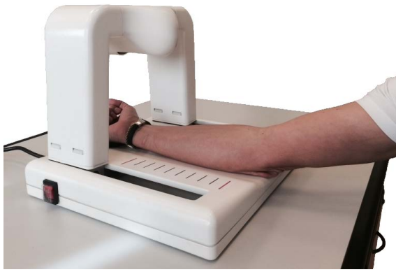
Fig. 2. Device for automated prick test reading developed at CEIT.
