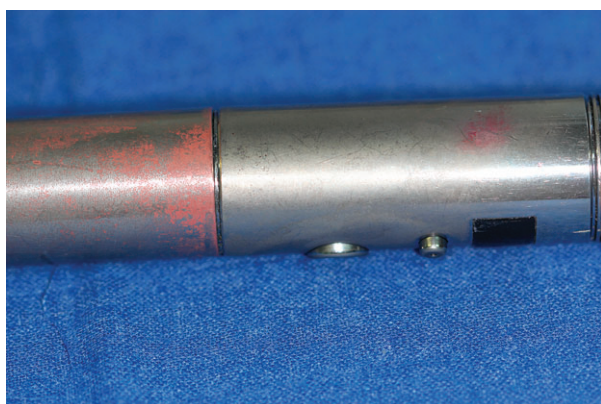
Fig. 4. Electronic cigarette corroded by the sweat of the hands of the patient.
