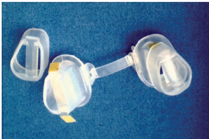
Fig. 1. Nasal air sampler with one of the nostril samplers assembled. The other nostril sampler shows the adhesive tape (with the yellow tabs at ends) and the silicone sleeve.
