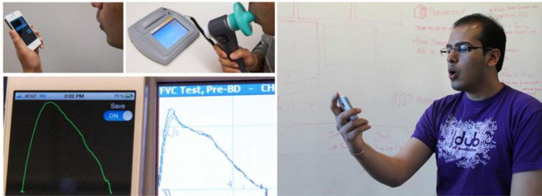
Fig. S1 Subjects using SpiroSmart (left) and a clinical spirometer (right) with their corresponding example curves. (The images have been downloaded from the websites http://www.medgadget.com/2012/09/spirosmart-iphone-app-accurately-estimates-lung-air-volume-video.html ; http://www.webpronews.com/spirosmart-app-turns-your-iphone-into-an-accurate-spirometer-2012-09 ; and http://ubicomplab.cs.washington.edu/wiki/SpiroSmart .)
