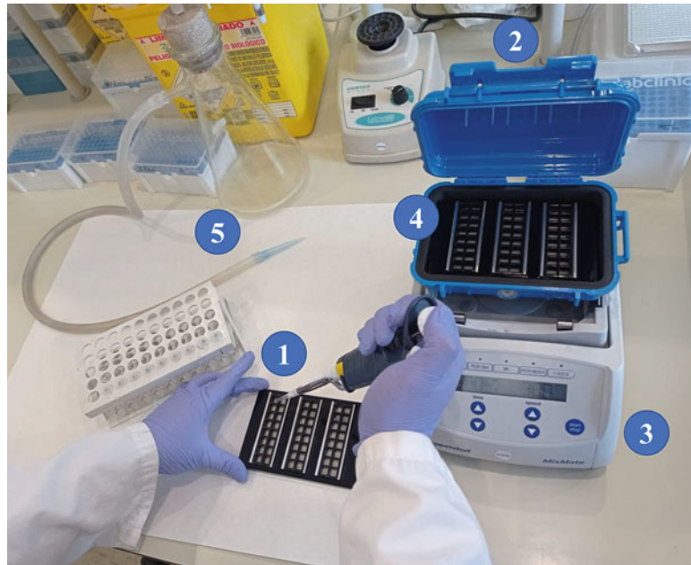
Fig. 3 Microarray hybridization: (1) multi-well incubation chamber, (2) microBOX™ incubation chamber, (3) orbital shaker, (4) multi-well incubation holder, (5) vacuum system for aspiration
